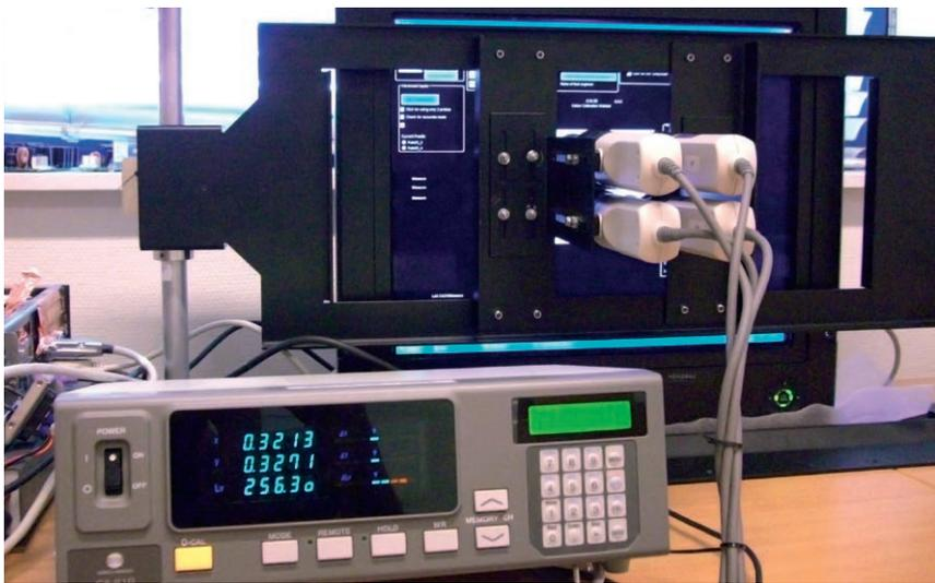
Hatteland Technology offers color calibration as either part of a complete Type Approved product delivery ready to be integrated straight into your systems, or as a support service to be utilized at any stage of your manufacturing and service processes. RS-232 / RS-422 / R-S485 is standard interface solution. Other solutions for communication between our MMD display and computer system are available as OEM / custom solution.
