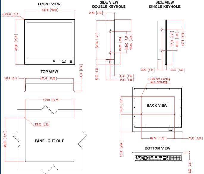
Dimensions might be shown with or without decimals and indicated as mm [inches]. Tolerance on drawings is +/- 1mm. For accurate measurements, check relevant DWG file.
