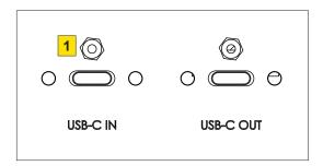
Illustration: USB-C Dasiy chaning, upto 3xFHD dispalys with touch. First display can be powered via USB-C.
