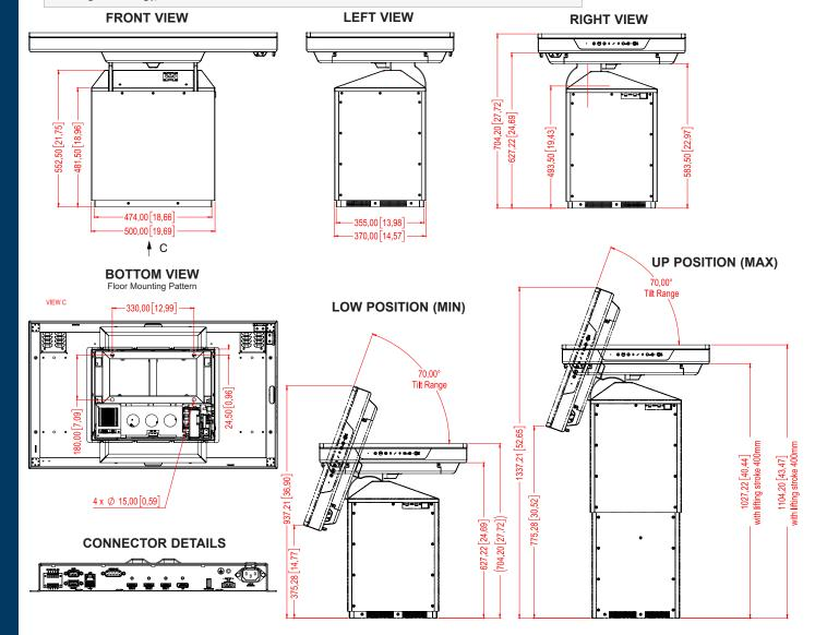
Dimensions might be shown with or without decimals and indicated as mm [inches]. Tolerance on drawings is +/- 1mm. For accurate measurements, check relevant DWG file.
