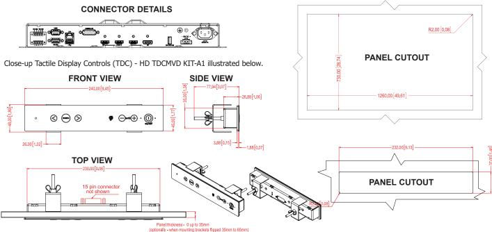
Dimensions might be shown with or without decimals and indicated as mm [inches]. Tolerance on drawings is +/- 1mm. For accurate measurements, check relevant DWG file.
