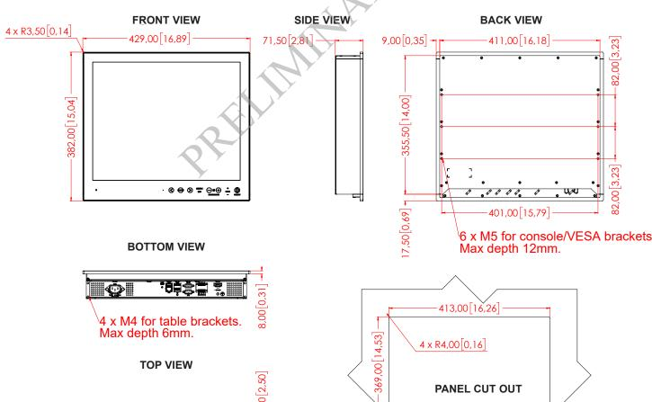
Dimensions might be shown with or without decimals and indicated as mm [inches]. Tolerance on drawings is +/- 1mm. For accurate measurements, check relevant DWG file.
