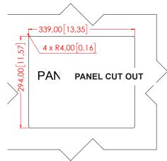
Dimensions might be shown with or without decimals and indicated as mm finches). Tolerance on drawings is +/- 1mm. For accurate measurements, check relevant DWG file
